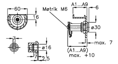
Door + frame thickness = 32-40 Measure type = A4
